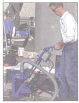
with standard sized machines. But it turns out that it can create deeper profiles as deep as  $^3/_{16}$  ths of an inch through stencils when that is desired. The tool is powered by 7-inch 110-volt angle
